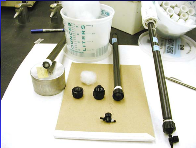
Ion exchange resin columns and hardware used to fill and extract the columns
