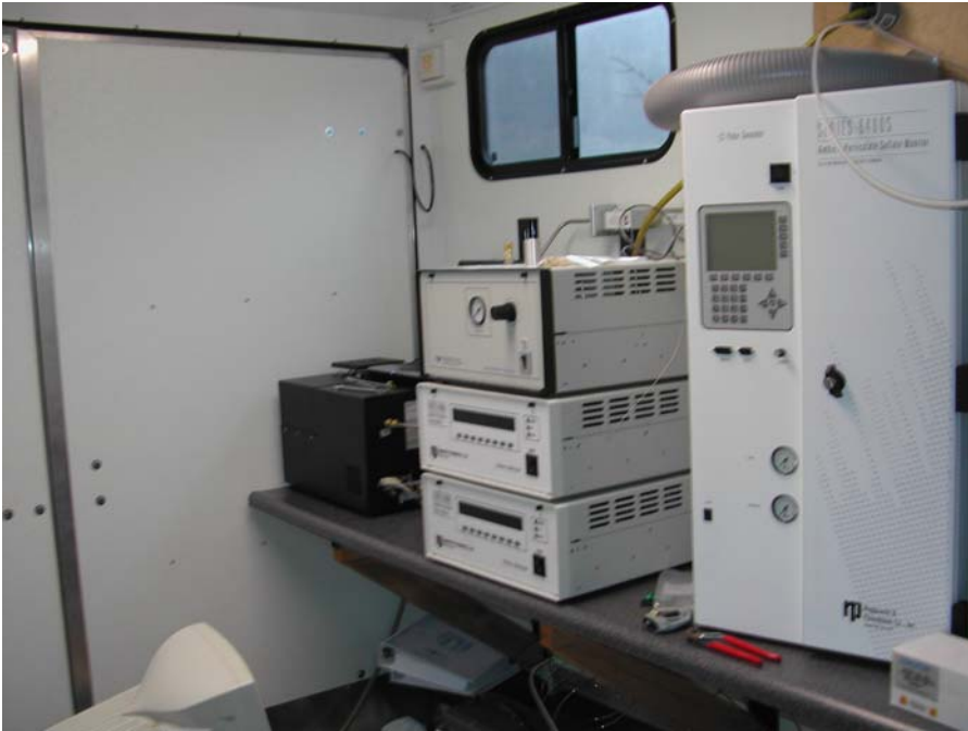
Sulfate pulse generator on right with zero air gas generator, sulfate, and nitrate analyzers in stack of three and the EC/OC analyzer on far left (black boxes) in trailer at Bonneville Dam
