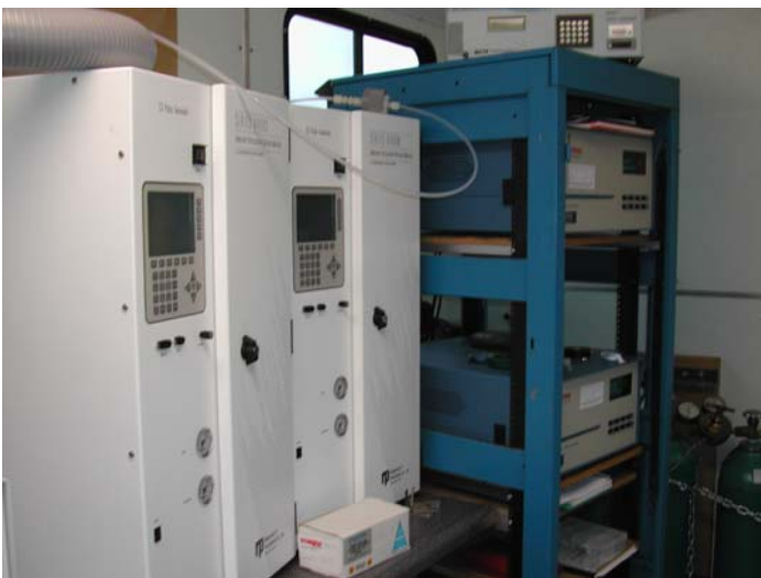
Sulfate and nitrate pulse generators on left with NO x and SO 2 monitors in blue rack in trailer at Bonneville Dam
