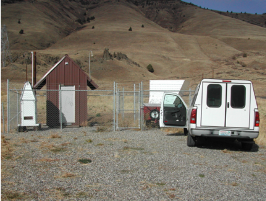
Towal road shelter (nephelometers and meteorological station) with IAS sampler in front of door on shelter and SODAR on right in front of pickup – IAS installed December 3, 2003. White shed on left was for former fluoride monitors.
